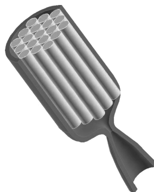
Fig. 4 Perspective view of the assembled Catuscia engine. All modules discharge in the same nozzle.
